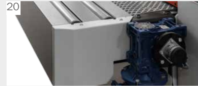
20 Variable speed conveyor belt drive Bandmotor Motovariateur tapis
